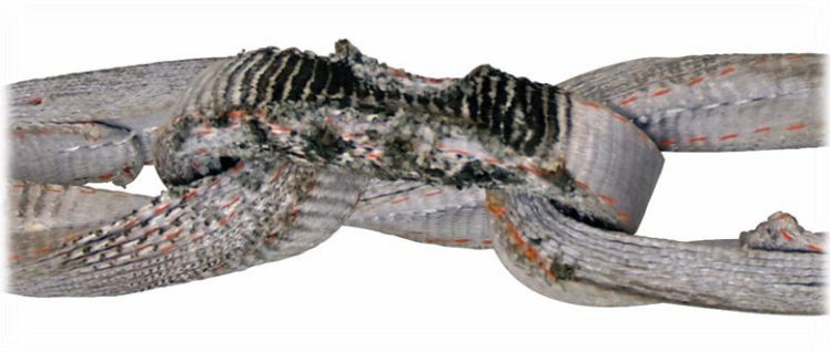
Fig. 6: Tissue damage due to heat exposure
