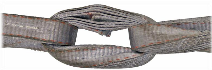
Fig. 5: Torn sewing on chain link
