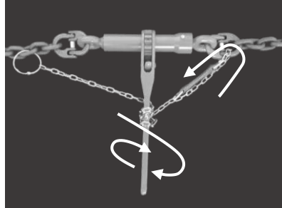
Fig. 7: How to use the safety chain
